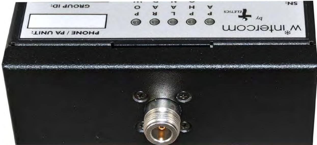
The **ANTENNA** connection is not labeled, and is by itself at the opposite end of the wintercom. It is for use with an antenna rated for 5.8GHz operation. Please contact your Teletics distributor for additional antenna and RF cable assemblies made to your requirements. This connector is a standard N Female.
